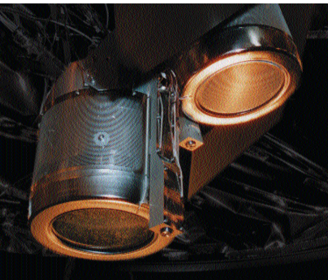
Figure 1. Xenon ion propulsion subsystem thrusters.
