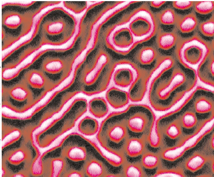
Figure 1. Bubbles and stripes in a 100-µm atomic force microscope image of an 8-µm-thick magnetic garnet film originally developed for magnetic bubble memories.
